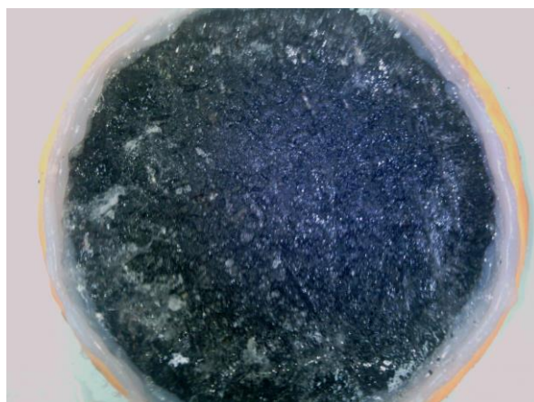
Figure 4. Test piece of the viscosity-reducing and ice-defending materials after 7 cycles of ball impact test.
