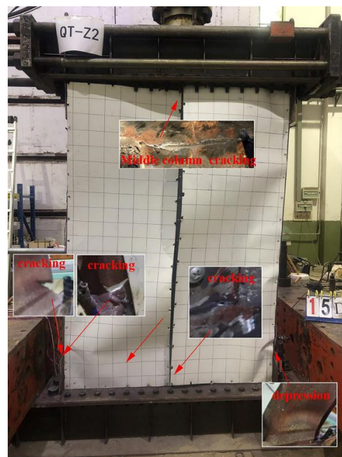
Figure 11. Failure image of QT-Z2.
