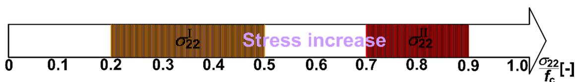
**Figure 2.** Ranges of the levels of critical stress  $\sigma_{22}^I$  and  $\sigma_{22}^{II}$  in ordinary concrete subjected to various material, technological, and service factors (according to [95]).
