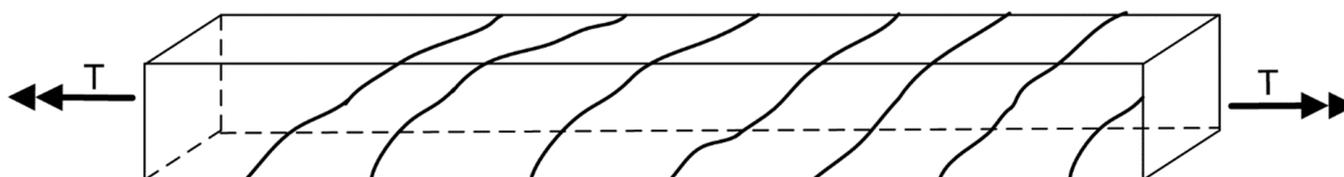
**Figure 8.** Macrocracks due to torsion;  $T$ —torsional moment.
