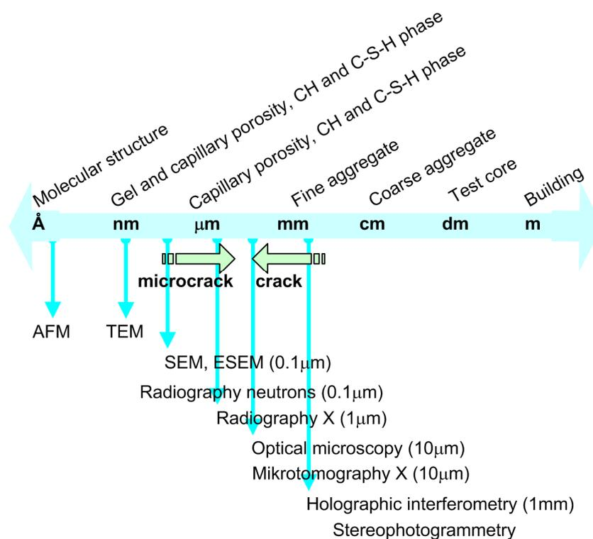
**Figure 11.** Methods for the detection of microcracks and cracks assigned to different scales of observation (according to [241]).
