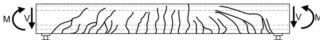
**Figure 7.** Macrocracks due to shear;  $M$ —as in Figure 5,  $V$ —shear force.
