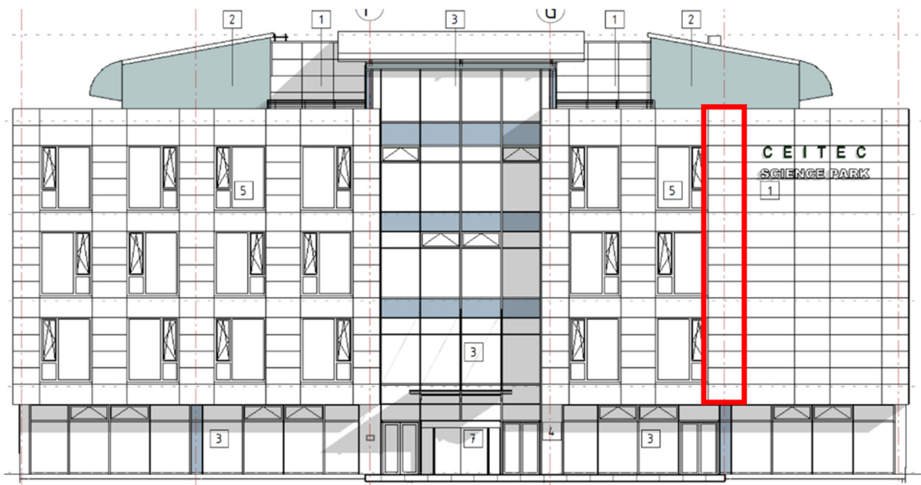
Figure 1. Measured and numerically evaluated faade. Façade part in question is marked red, façade height as well as air gap is approx. 13.7 m.
