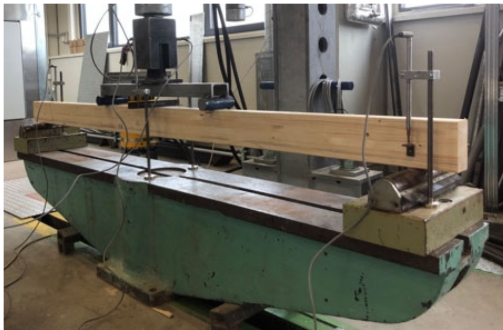
Figure 5. Test of the GLT testing body in the four-point bending test (authors' archive).
