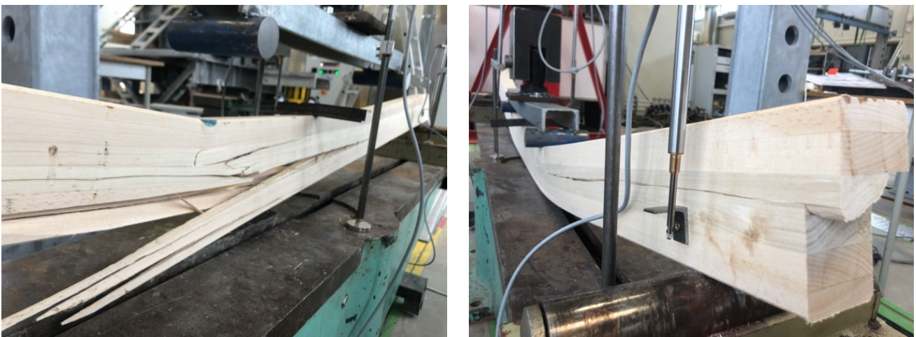
Figure 9. Examples of failure of the hybrid beech–poplar beam (BE-PO (hyb)) (authors' archive).
