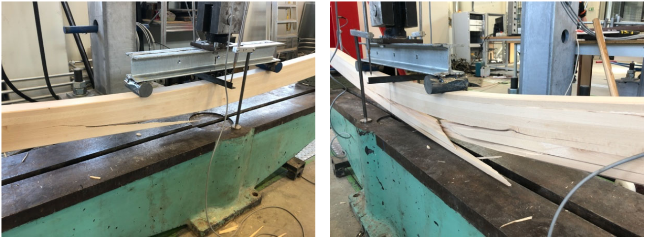
Figure 8. Examples of failure of the homogeneous beech beam (BE (h)) (authors' archive).
