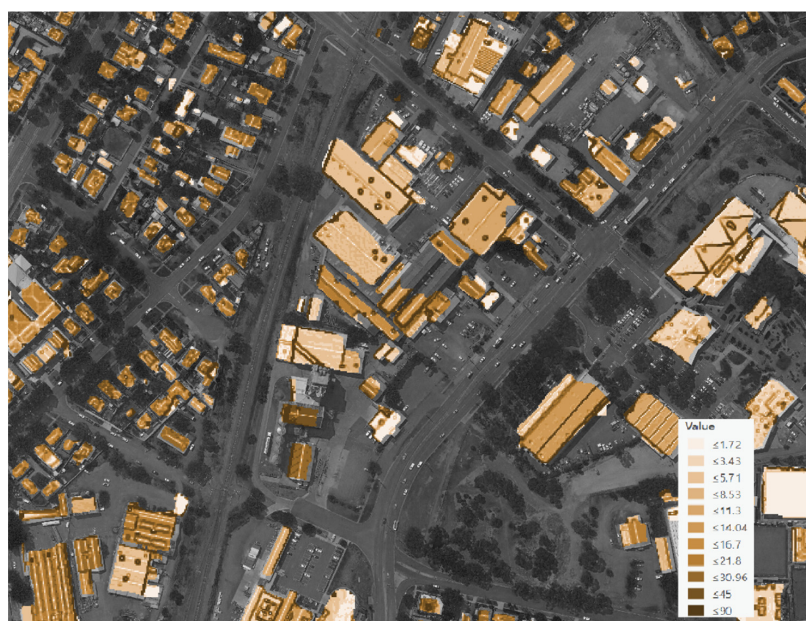
Figure 4. Roof tilt angle raster layer calculated using BHM and QGIS Slope function.
