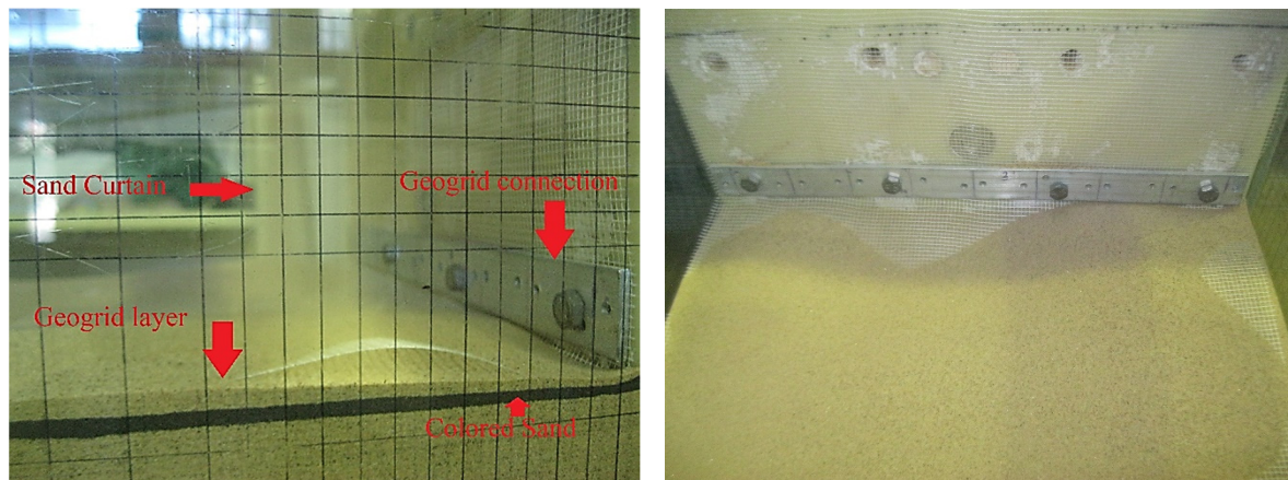
Figure 8. Pluviation and geogrid connection to the wall.
