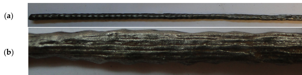
Figure 5. The sample \phi 6 (B500 B) after corrosion in corrosion chamber: (a) whole sample, (b) detail.
