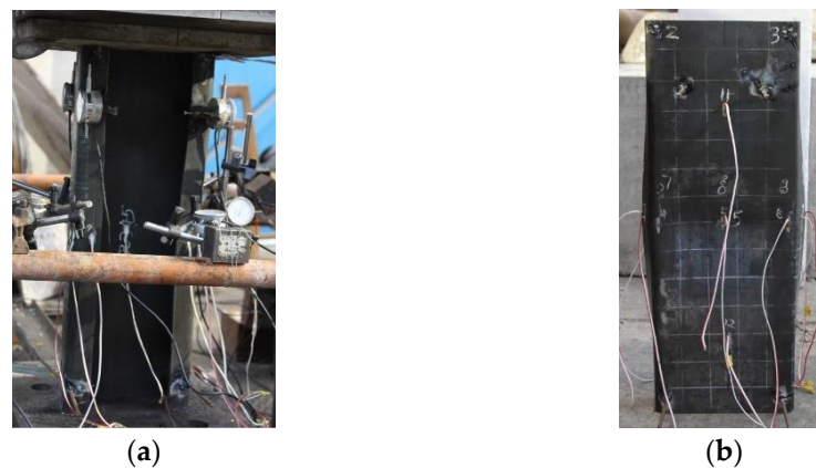
Figure 12. Failure mode of ZC3: (a) ultimate failure state; (b) final failure mode.
