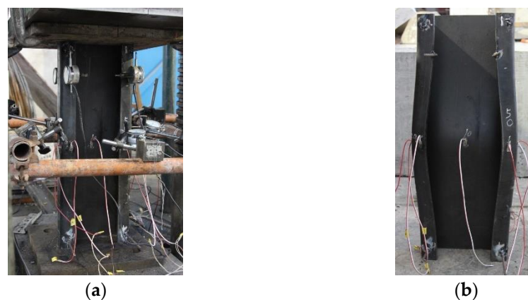
Figure 11. Failure mode of ZC2: (a) ultimate failure state; (b) final failure mode.
