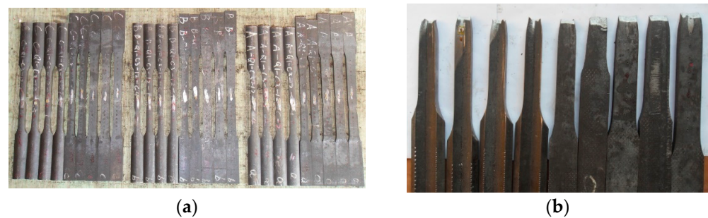
Figure 4. Specimen fractures: (a) overall fracture; (b) part fracture.
