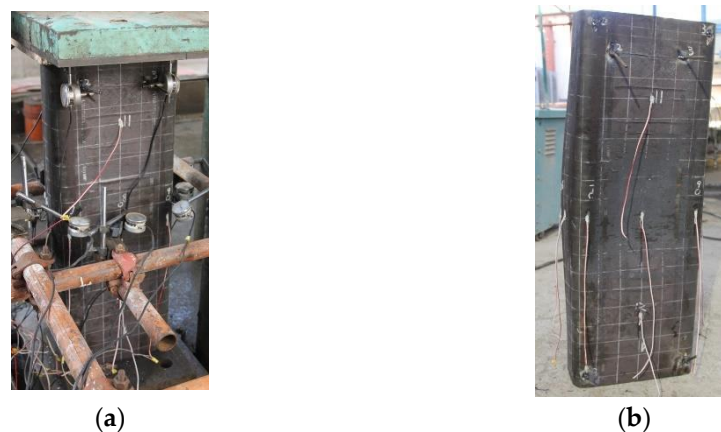
Figure 14. Failure mode of ZC5: (a) ultimate failure state; (b) final failure mode.
