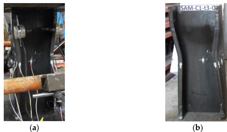
Figure 10. Failure mode of ZC1: (a) ultimate failure state; (b) final failure mode.
