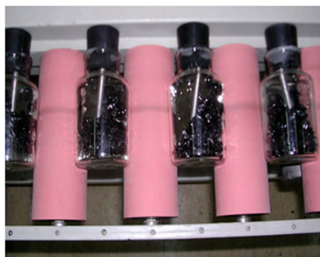
Figure 5. Dynamic water immersion test.
