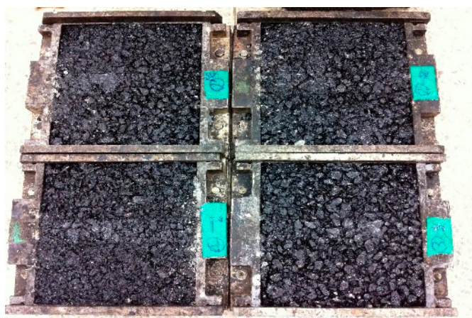
Figure 16. Specimen after wheel tracking test.
