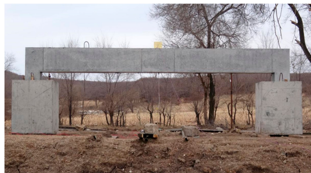
Figure 3. Layout of beam specimen after construction.
