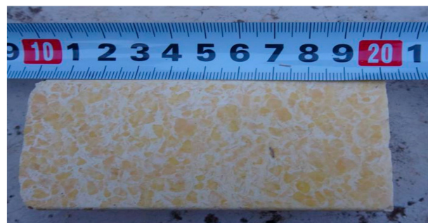
(a) Dimension of single TNT explosive block.
