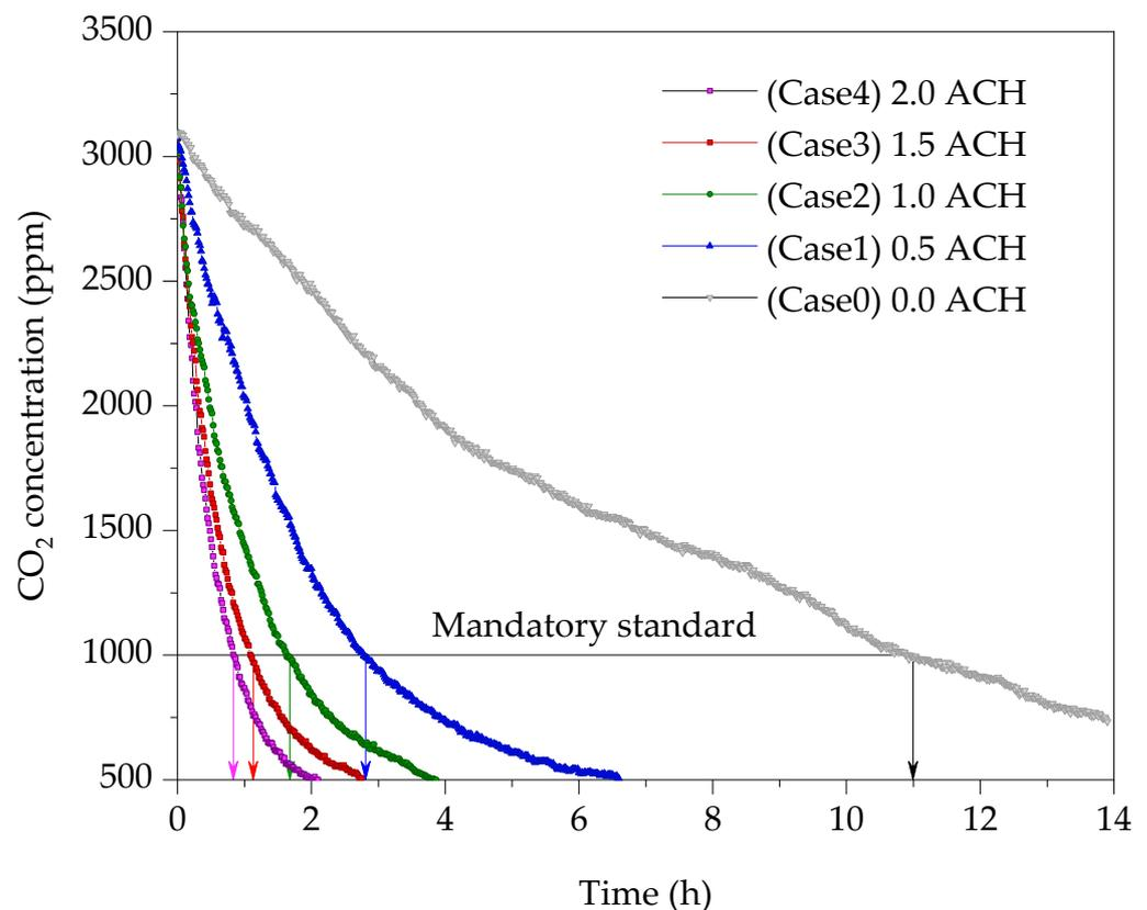
**Figure 6.** The concentration changes of indoor CO<sub>2</sub> due to operating mechanical ventilation systems with different air change rates.
