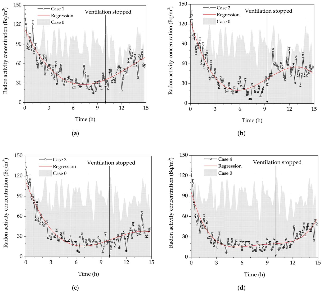
**Figure 8.** The concentration changes of indoor radon activity due to operating mechanical ventilation system with different air change rates: (a) Case 1—0.5 ACH; (b) Case 2—1.0 ACH; (c) Case 3—1.5 ACH; (d) Case 4—2.0 ACH.
