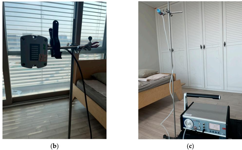
**Figure 3.** The measurements in R2: (a) measurement point; (b) EE820 sensor for CO<sub>2</sub>; (c) AlphaGUARD DF2000 for radon.
