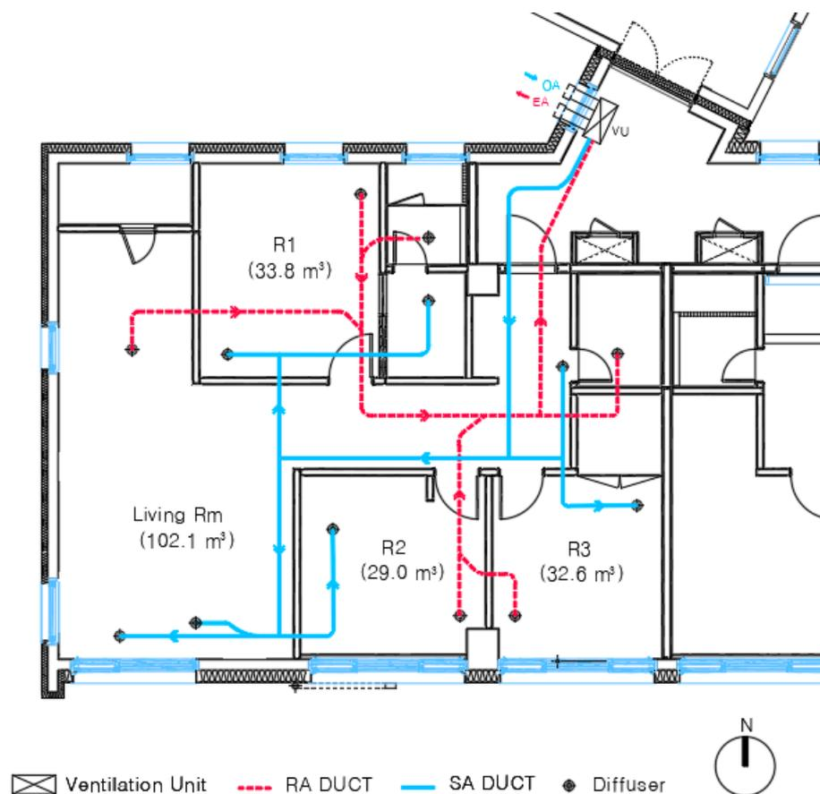
**Figure 1.** The duct work plan of the apartment and the subject space (R2) for the experiments.
