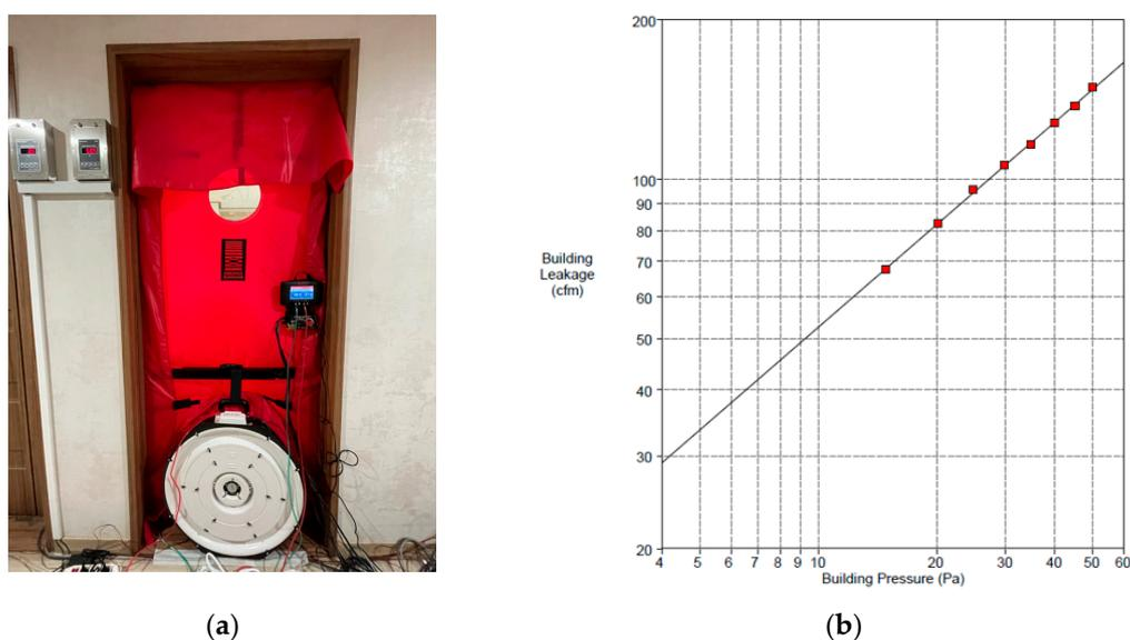
**Figure 5.** The blower door test result of the R2: (a) a setup of the blower door test equipment; (b) blower door test result graph.
