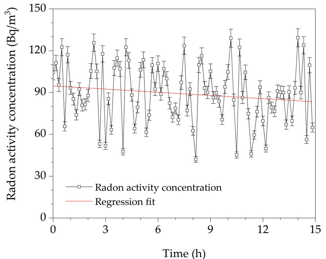
**Figure 7.** The temporal variation of indoor radon activity concentration in R2 without ventilation (Case 0).
