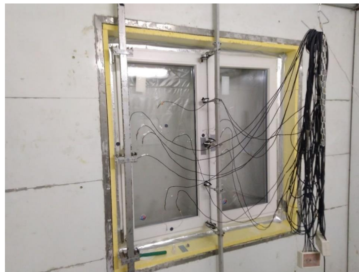
Figure 4. PVC window installed in a climate chamber for temperature deformation tests.
