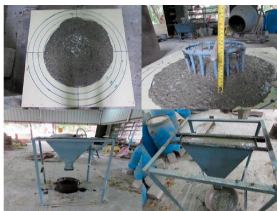
Figure 2. View of workability tests of fresh SCC.
