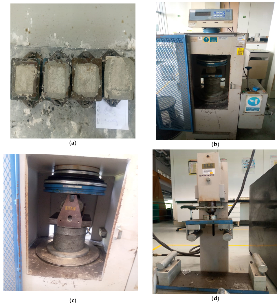
Figure 1. (a) Sample preparation, Equipment for testing of (b) CS (c) STS (d) FS.
