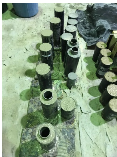
Figure 8. Supporting the columns using wood plates before casting.
