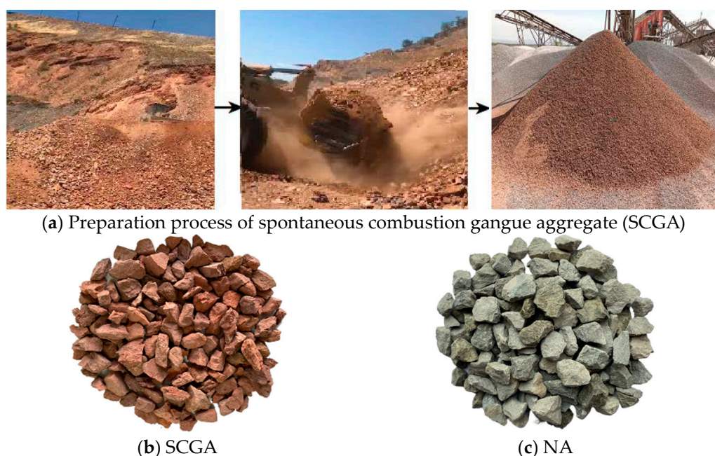
Figure 1. (a) Preparation process of spontaneous combustion gangue aggregate (SCGA); (b) SCGA; (c) natural aggregates (NA).
