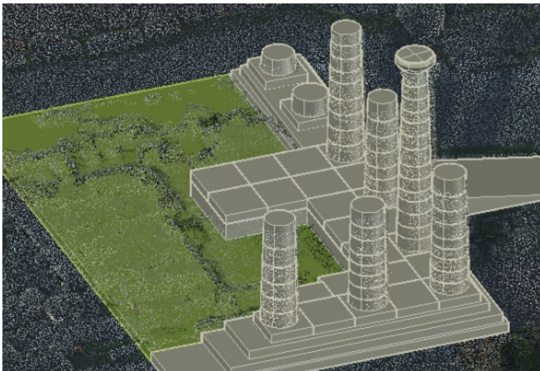
Figure 4. Comparison of CAD model with initial 3D point cloud.
