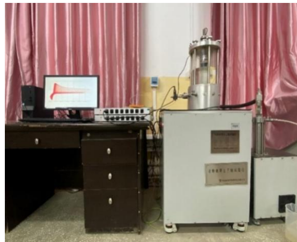
Figure 2. KTL-DYN10 dynamic triaxial equipment.
