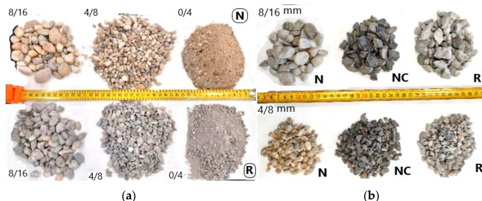
**Figure 1.** (a) Illustrates the distinction between natural (N) and recycled (R) fine and coarse aggregates, (b) Coarse aggregates: Natural (N), Crushed Stone (NC), and Recycled (R).
