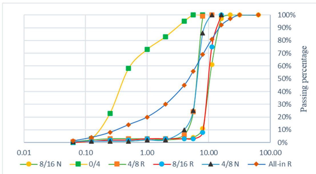
**Figure 3.** Grading curves of the fine and coarse aggregates.
