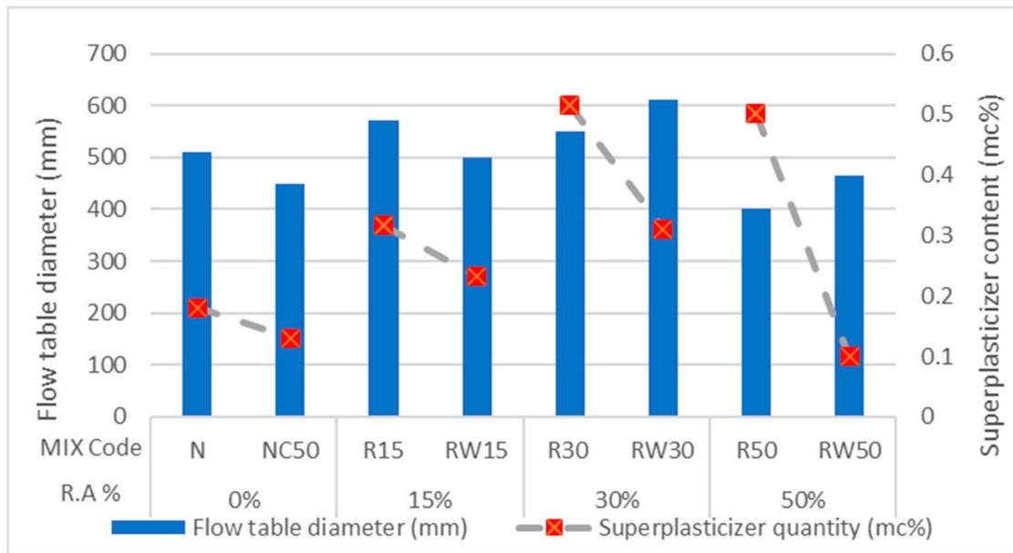
**Figure 4.** Flow table results and superplasticizer content for both the dried and partially saturated conditions of recycled aggregates.
