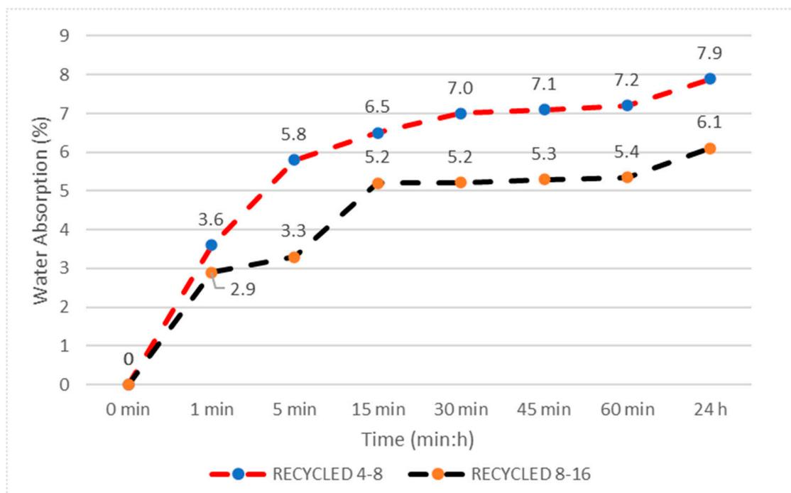
**Figure 5.** Water absorption of recycled aggregate over 24 h period.
