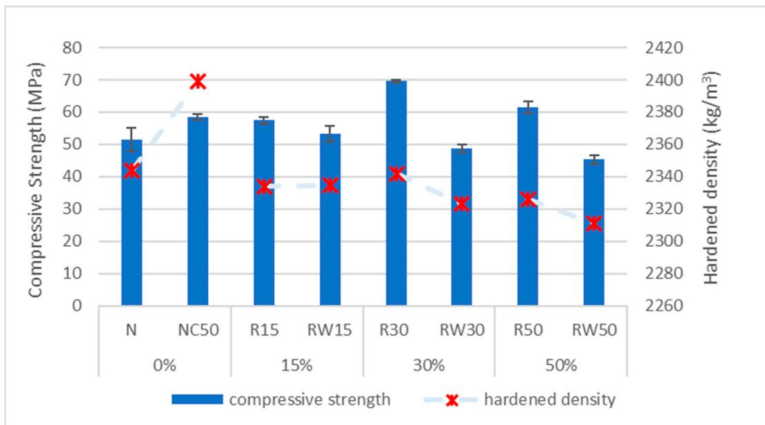
**Figure 7.** The compressive strength and the hardened density results (average values and ranges).
