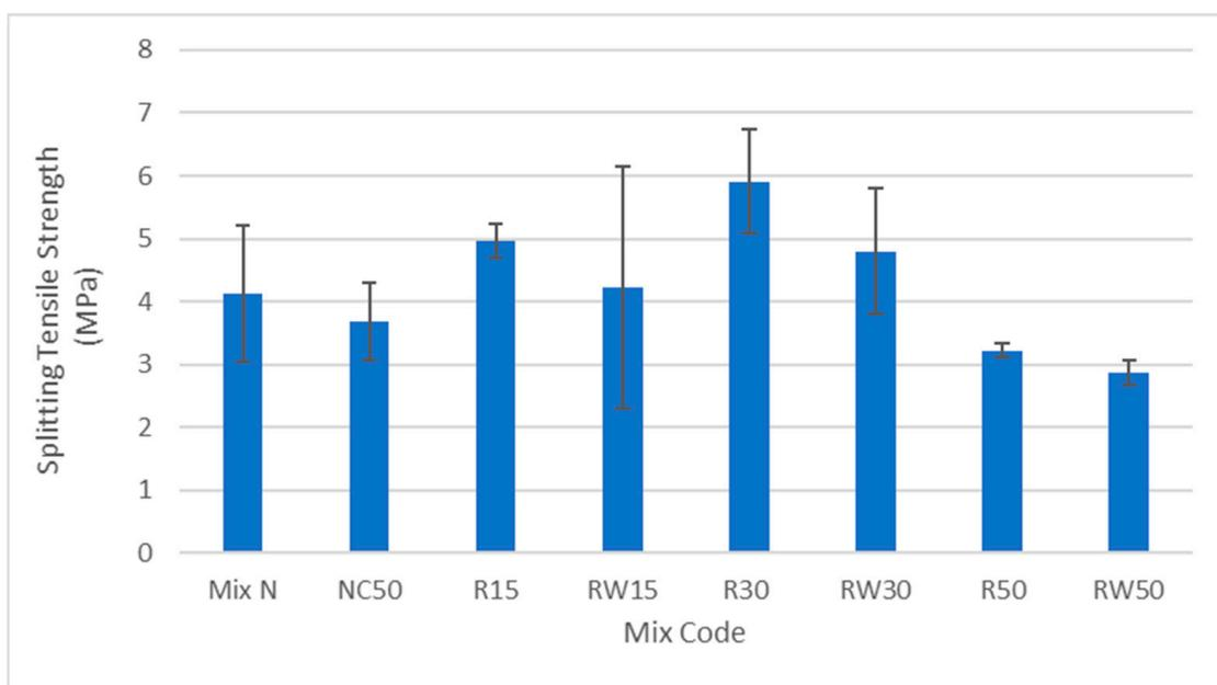
**Figure 8.** Splitting tensile strength results (average values and ranges).
