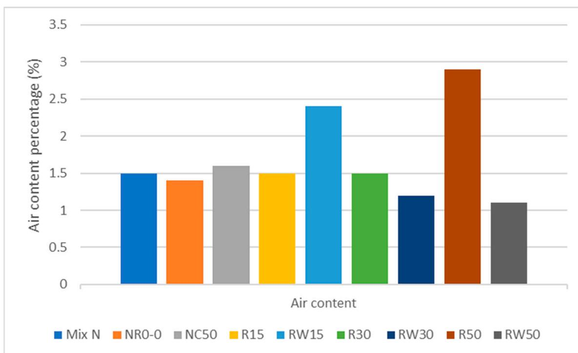
**Figure 6.** Air content results of fresh concrete.
