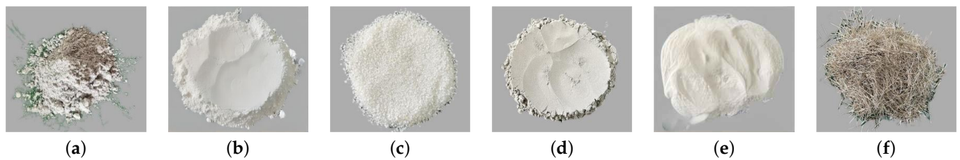
Figure 3. Material used to form UHPC: (a) Cement; (b) Silica fume; (c) Quartz sand; (d) Fly ash; (e) Water reducer; (f) Fiber.
