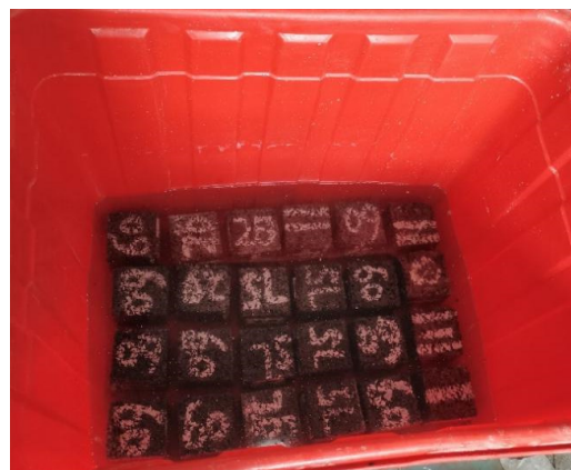
Figure 5. The acid corrosion of specimen.
