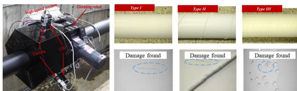
Figure 7. Climbing robot and the damage detection under three suspender surface types [37].
