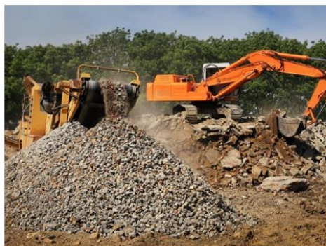
(a) Waste Concrete Crushing and recycled aggregate (b) Use of manufactured aggregate for road construction
