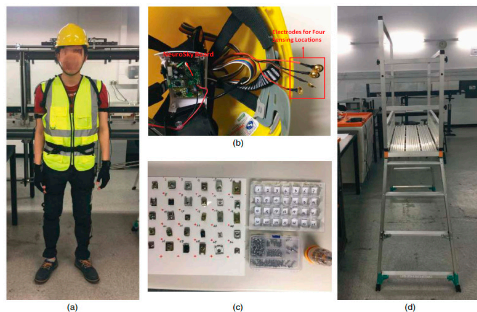
Figure 4. Experimental apparatus: (a) experiment subject; (b) EEG hardhat and the EEG monitoring chips; (c) nuts and bolts; (d) ladder platform [51].
