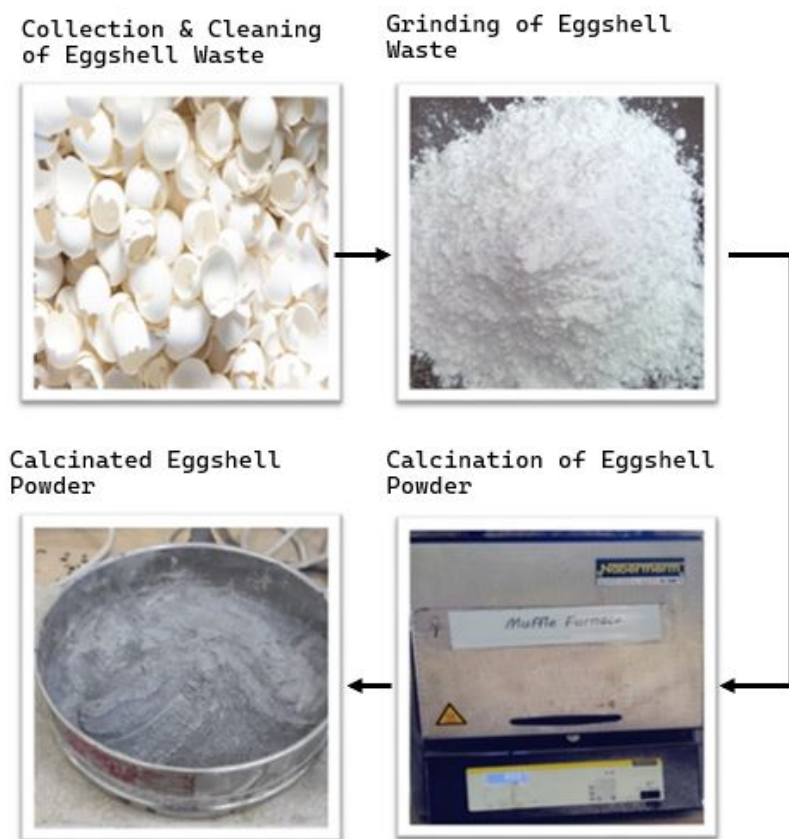
Figure 1. Converting eggshell waste to treated eggshell powder [16].
