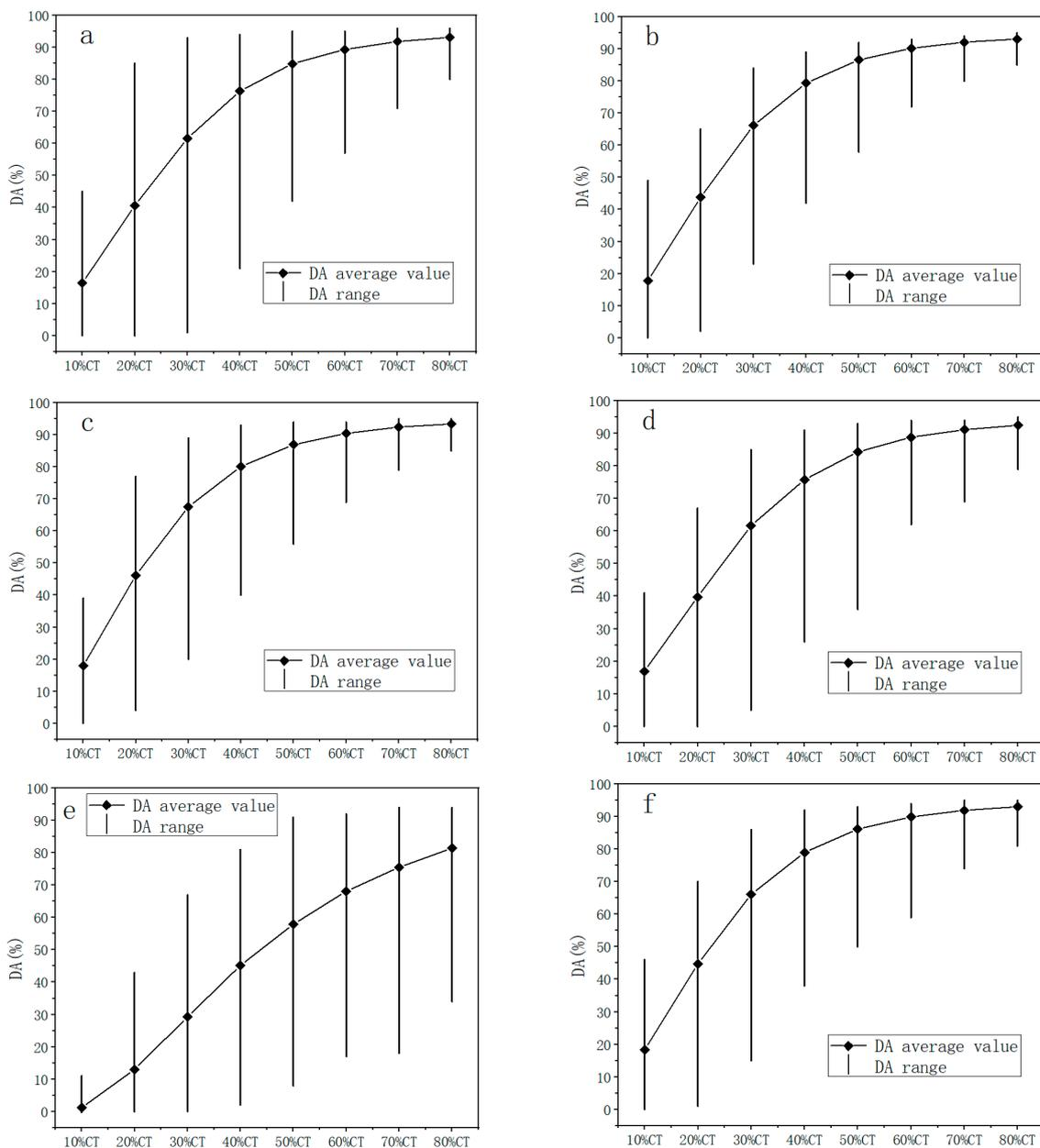
**Figure 5.** DA curves of six kinds of skylight: (a) centralized rectangular skylight; (b) distributed rectangular skylight; (c) centralized ribbon skylight; (d) distributed vertical strip skylight; (e) centralized X-shaped skylight; (f) distributed horizontal strip skylight.
