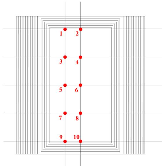
**Figure 8.** Distribution of measuring points for indoor illuminance (Points 1–10).
