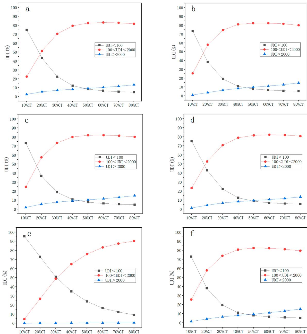
**Figure 7.** UDI curves of six kinds of skylight: (a) centralized rectangular skylight; (b) distributed rectangular skylight; (c) centralized ribbon skylight; (d) distributed vertical strip skylight; (e) centralized X-shaped skylight; (f) distributed horizontal strip skylight.
