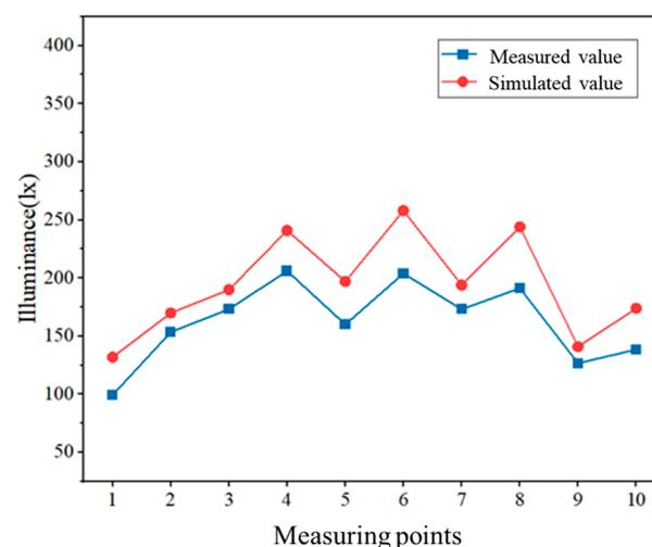
**Figure 9.** Comparison of illuminance measurement values with simulation.
