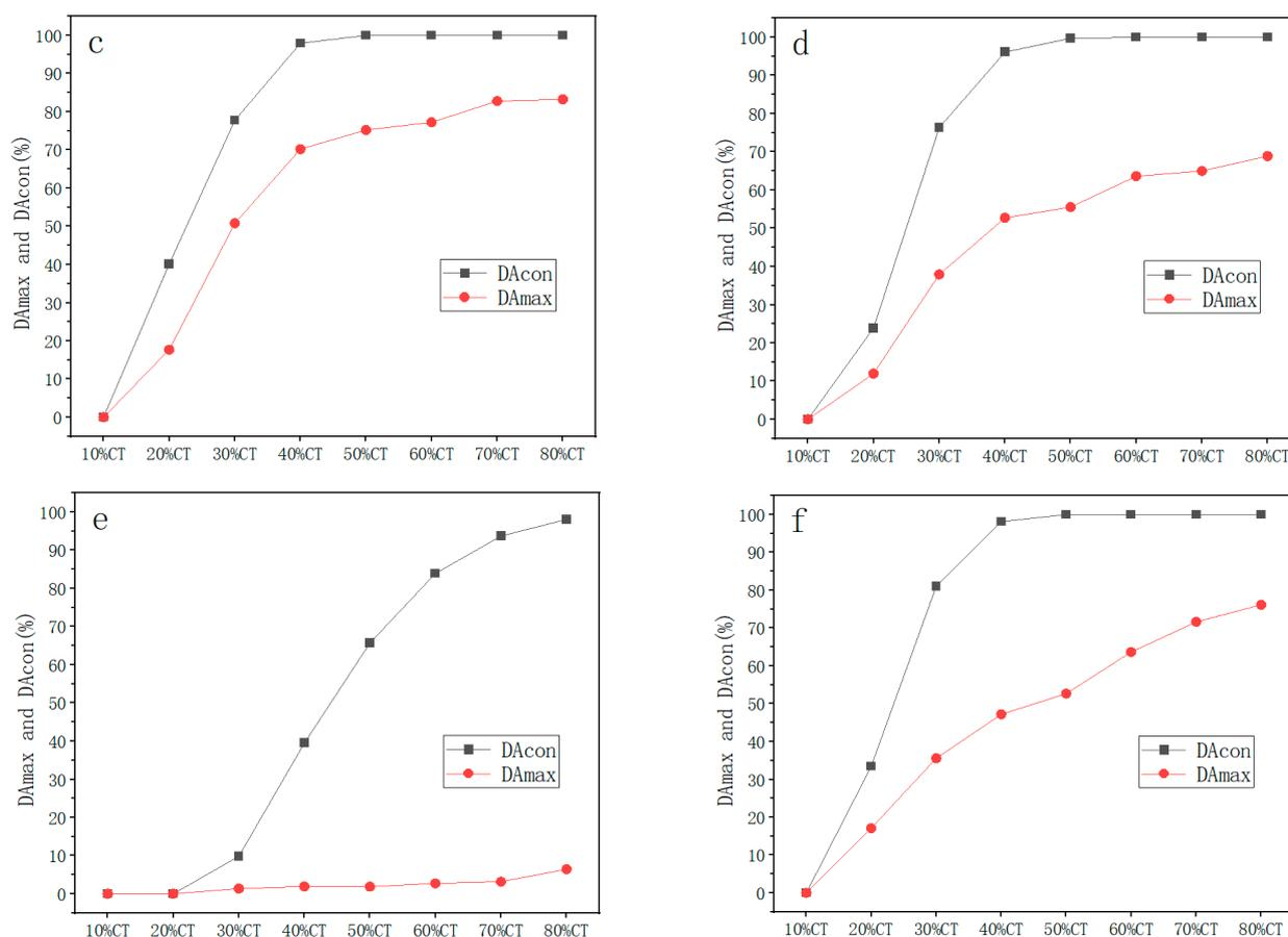
**Figure 6.** DAcon and DAmix curves of six kinds of skylight: (a) centralized rectangular skylight; (b) distributed rectangular skylight; (c) centralized ribbon skylight; (d) distributed vertical strip skylight; (e) centralized X-shaped skylight; (f) distributed horizontal strip skylight.
