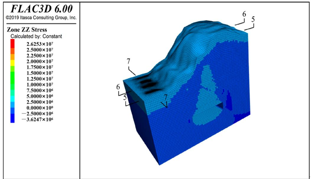
**Figure 20.** Vertical stress diagram after coal mining. 5-5, 6-6, and 7-7 indicate the profile direction.
