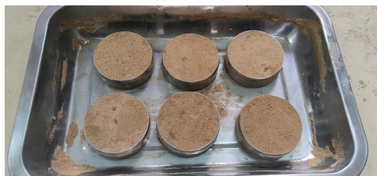
(b) Expanded soil specimen
