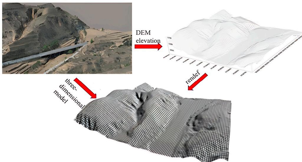
Figure 10. Three-dimensional surface of bridge area.
