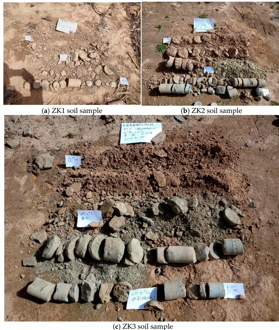
**Figure 3.** Drilling core soil samples. The Chinese characters in the figure only indicate the depth and type of rock samples, which has little influence on the research content of this paper.
