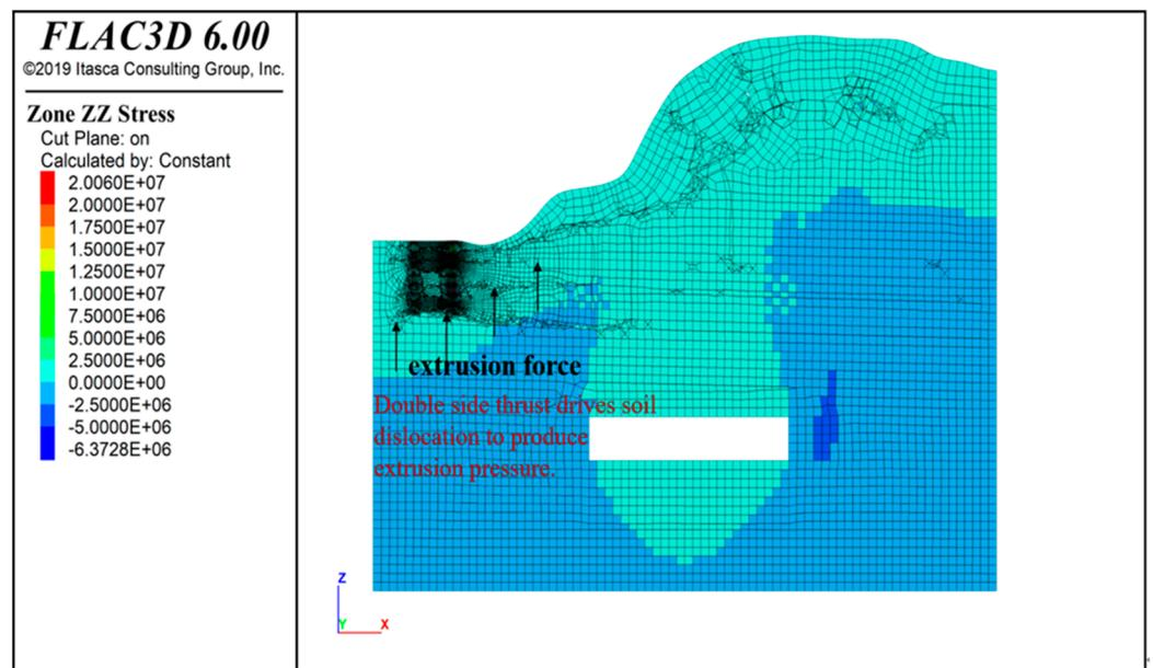
Figure 22. 6-6 vertical stress diagram (X-Z).
