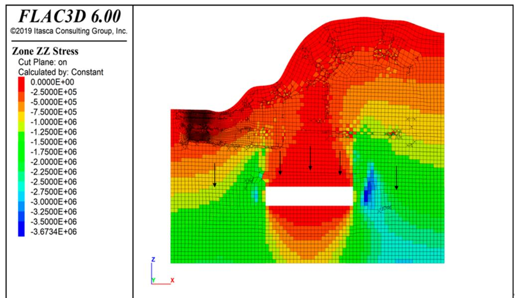
**Figure 21.** 5-5 vertical stress diagram (X-Z). The arrows in the figure represent the gravity of the overlying soil. The white part in the figure is the part of simulated underground goaf.
