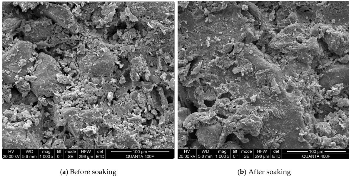
**Figure 4.** Micro-particle morphology of soil samples before and after soaking (1000 times).
