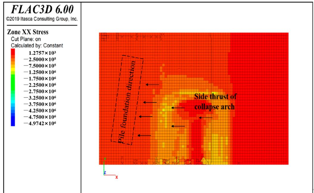
Figure 18. 3-3 horizontal stress diagram.
