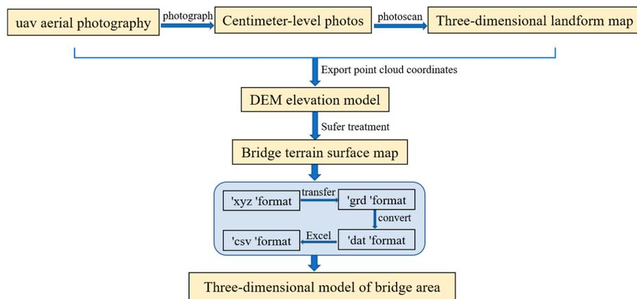
**Figure 9.** Flow chart of 3D model establishment.
