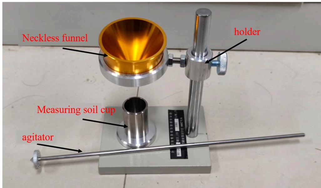
(a) Free expansion rate measuring instrument
