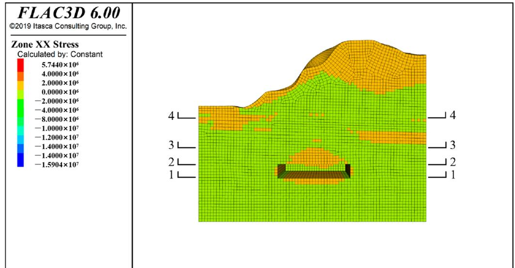
Figure 15. Horizontal stress diagram after coal mining. 1-1 indicates the cross section.
