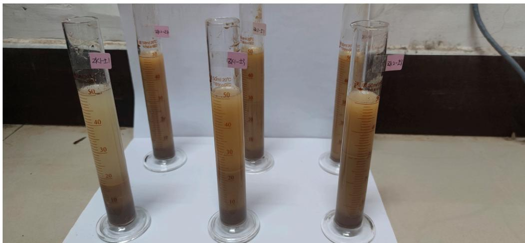
(b) The measuring cylinder is stationary for 24 h
