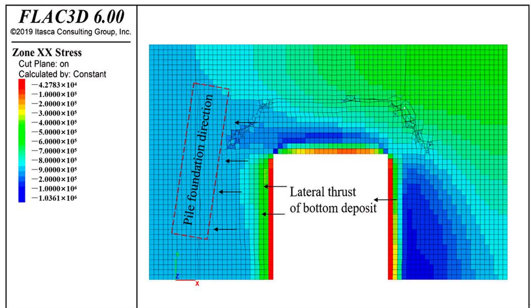
Figure 16. 1-1 horizontal stress diagram.
