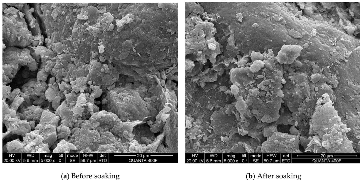
**Figure 5.** Micro-particle morphology of soil samples before and after soaking (5000 times).
