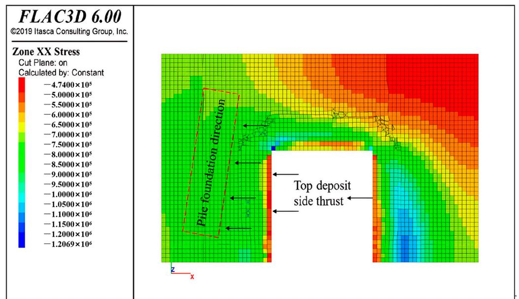
Figure 17. 2-2 horizontal stress diagram.
