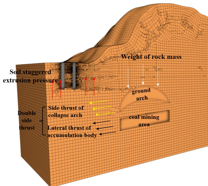
Figure 24. Schematic diagram of pile foundation uplift mechanism.
