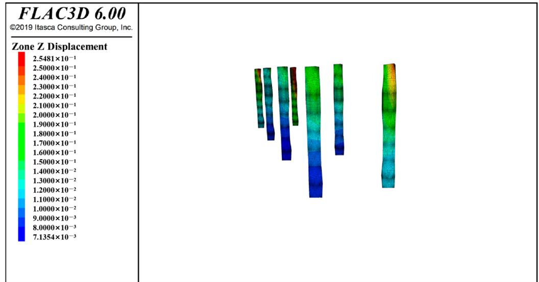
Figure 14. Displacement field of pile foundation after coal mining.
