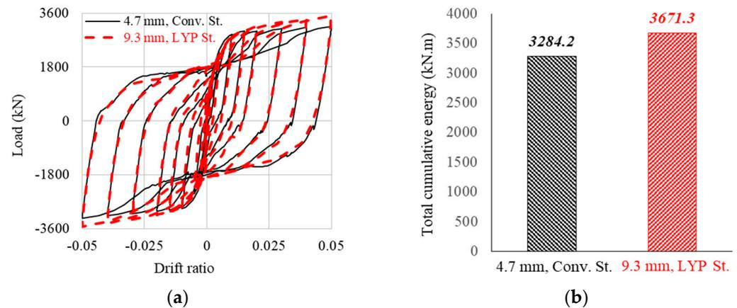
**Figure 9.** Comparison of cyclic performances. (a) Hysteretic behaviors; and (b) energy dissipation capacities.
