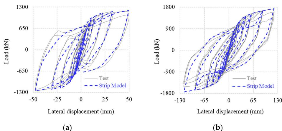
**Figure 11.** Comparison of the test results and strip model predictions. (a) Specimen no. 1 [16]; and (b) the SC2T specimen [19].
