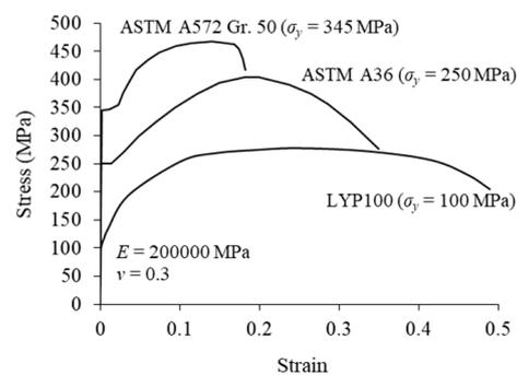
**Figure 2.** Properties of the adopted steel material.
