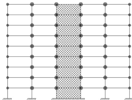
**Figure 10.** Interior gravity frame from the Los Angeles 9-story SAC building coupled with an SPSW system. (Note: 5 bays @ 9.144 m and 9 stories @ 3.9624 m).
