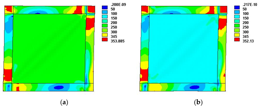
**Figure 8.** Comparison of stress contours and yielding patterns at 0.02 drift ratio. (a) 4.7 mm, conventional steel (original); and (b) 9.3 mm, LYP steel (retrofitted).
