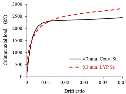
**Figure 7.** Comparison of axial loads in columns.
