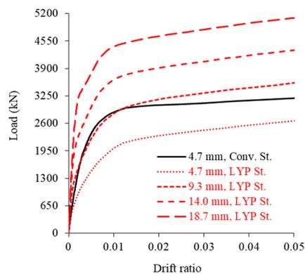
**Figure 5.** Load–drift responses of SPSWs with original and replaced infill plates.
