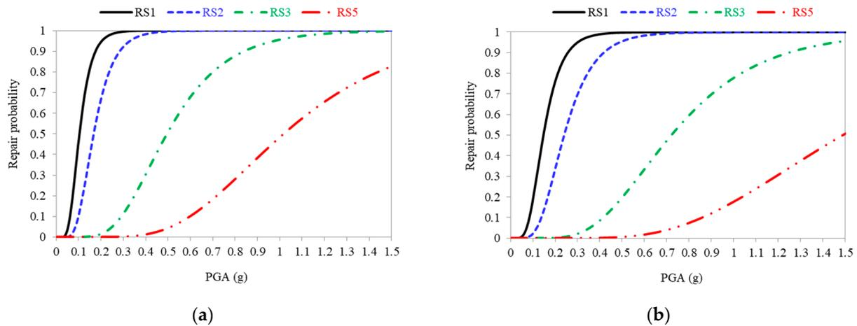
**Figure 13.** SPSW fragility curves. (a) Original; and (b) retrofitted.
