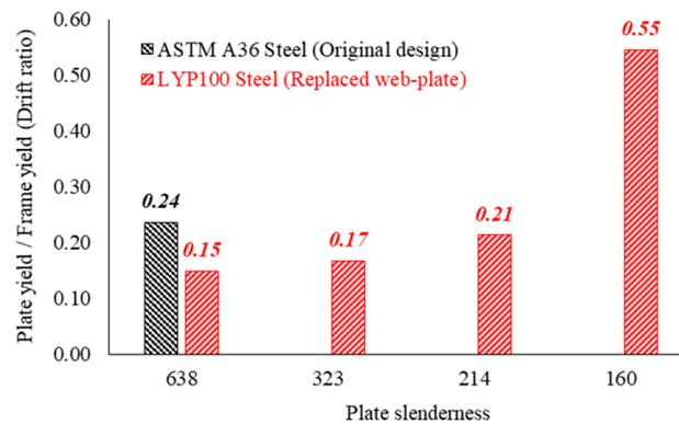
**Figure 4.** Initial plate and frame yieldings in SPSWs with original and replaced infill plates.
