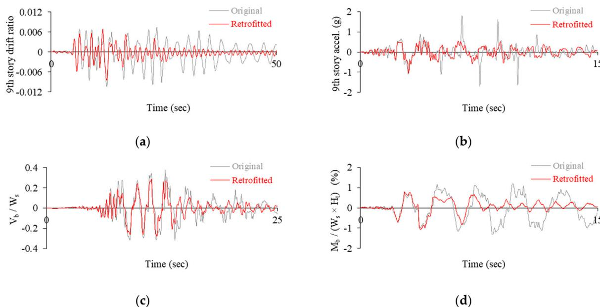
**Figure 12.** Comparison of the time histories of some seismic response parameters. (a) The 9th story drift ratio; (b) 9th story acceleration; (c) base shear; and (d) base moment.
