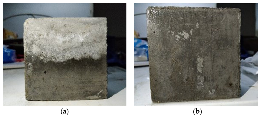
Figure 7. Appearance of concrete specimens in the semi-immersion drying test and full-immersion drying test: (a) salt crystals precipitated from semi-immersion drying test pieces, and (b) no salt crystals precipitated from the test piece after full-immersion drying.
