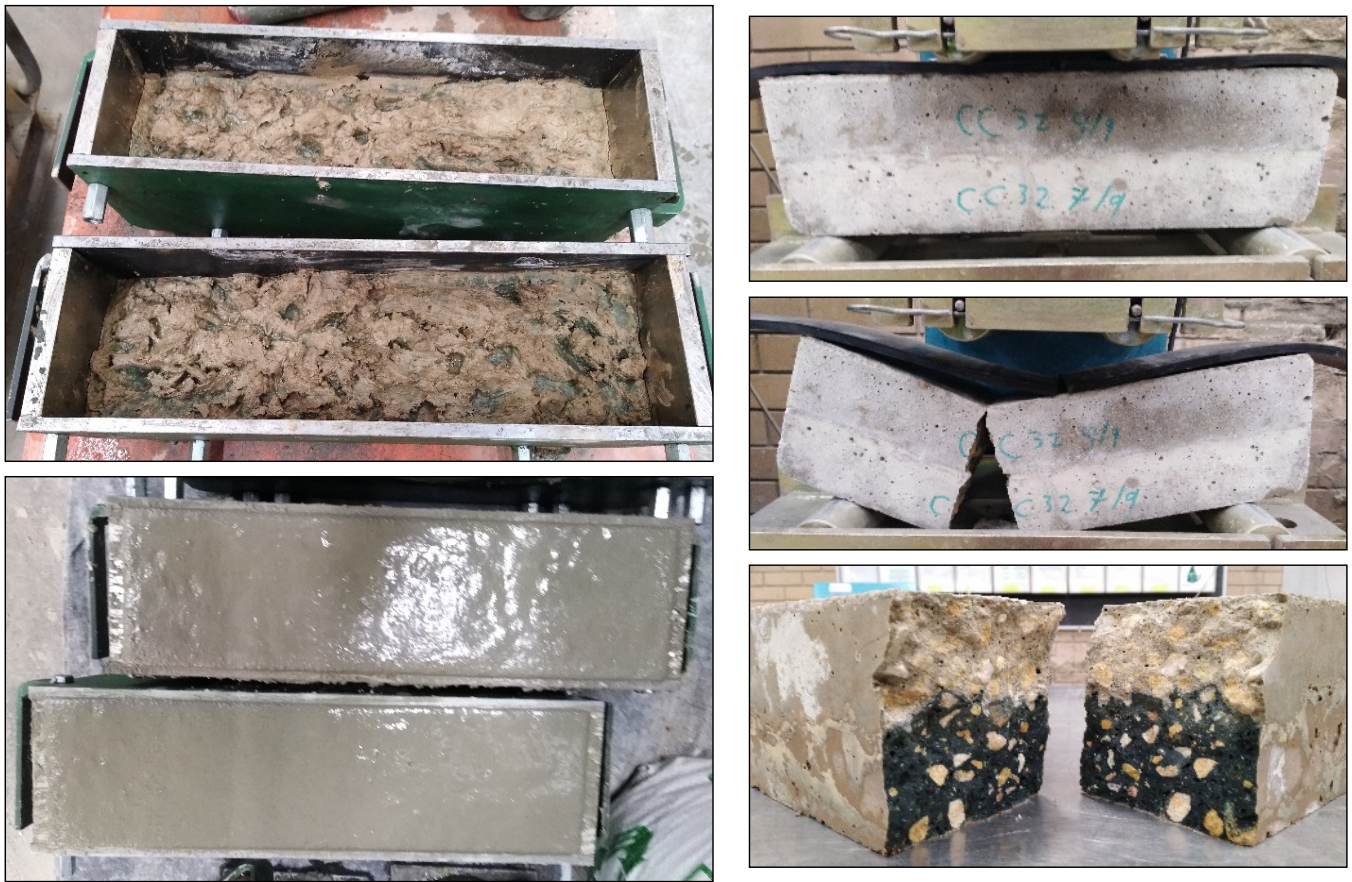
Figure 4. Preparation and testing of concrete joints in beams subjected to bending.
