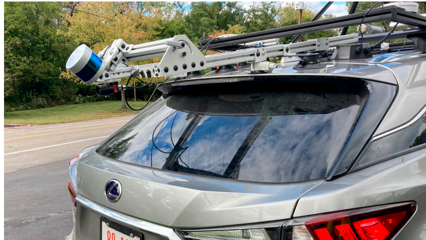
Figure 1. LiDAR data collection system.
