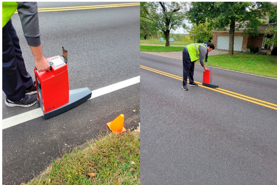
Figure 2. Manual measurement using a LTL-X handheld retroreflectometer.
