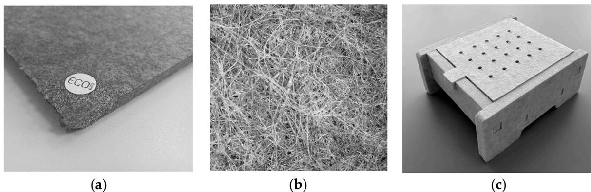
**Figure 1.** Eco-friendly acoustic panel: (a) rectangular sample of the fabricated material; (b) image taken with SEM for inspection of the fibrous microstructure; and (c) picture of the rectangular-shaped box designed for the cell viability assay.
