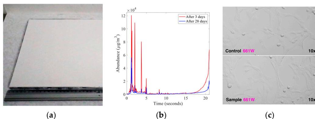
**Figure 3.** Results of the biocompatibility tests: (a) sample of material with no specimens identified after antifungal resistance test; (b) chromatography of the VOC emission test after 3 days (red line) and after 28 days (blue line); and (c) optical microscopy images (10 $\times$ ) of the 661W cell line seeded at a density of 100,000 cells per flask of the 661W line in (Top) control and (Bottom) sample conditions.
