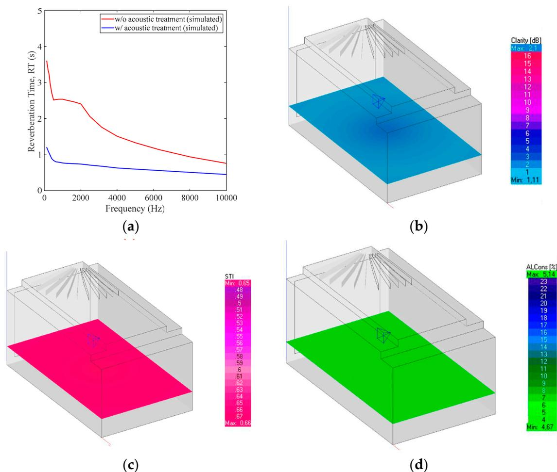
**Figure 8.** Noise pollution reduction and improvement of acoustic comfort in Case Study II: (a) Comparison of the predicted RT for the configurations without acoustic treatment (continuous magenta line) and with acoustic treatment (continuous cyan line); (b) C50; (c) STI; and (d) %Alcons distribution over the useful space.
