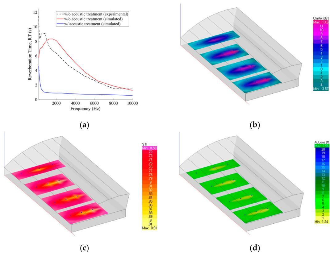
**Figure 6.** Noise pollution reduction and improvement of acoustic comfort in Case Study I: (a) comparison of the experimental (discontinuous black line) and predicted RT for the configurations without acoustic treatment (continuous red line) and with acoustic treatment (continuous blue line); (b) C50; (c) STI; and (d) %Alcons distribution over the useful space (areas most frequented by the alleged patients and healthcare workers).
