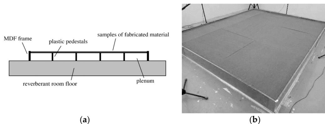
**Figure 2.** Sound absorption tests of the material under study: (a) schematic representation of the setup used for measurements with the plenum following ISO 10534-2; and (b) detailed view of the samples arranged for the tests in the reverberant chamber.
