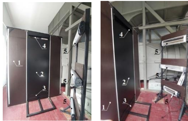
Figure 5. Photo of the experimental installation. Illustration by the authors. 1—external protection, 2—trombe shaft, 3—closed regulating valves, 4—own control valves, 5—infrared getter.
