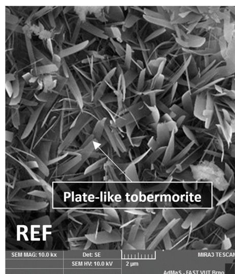
Figure 12. SEM image of reference sample autoclaved for 8 h with isothermal dwelling at 190 °C.
