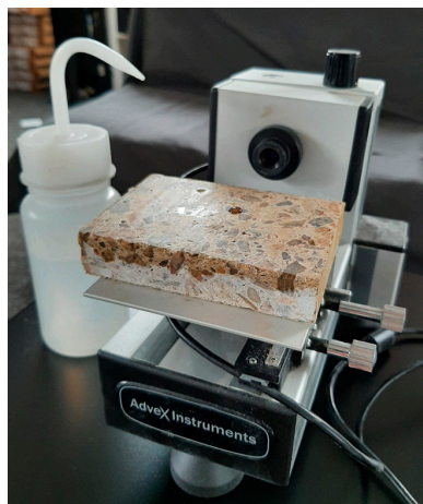
Figure 3. CCD camera for measuring the contact angle and surface energy of the hydrophobised surface.
