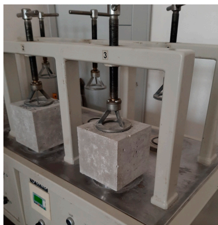
Figure 5. S1 samples treated by the hydrophobisation in the apparatus for the determination of the depth of penetration of water under pressure.
