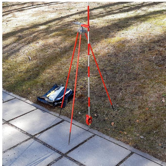
**Figure A2.** Mini prism and tripod used during total station surveys.
