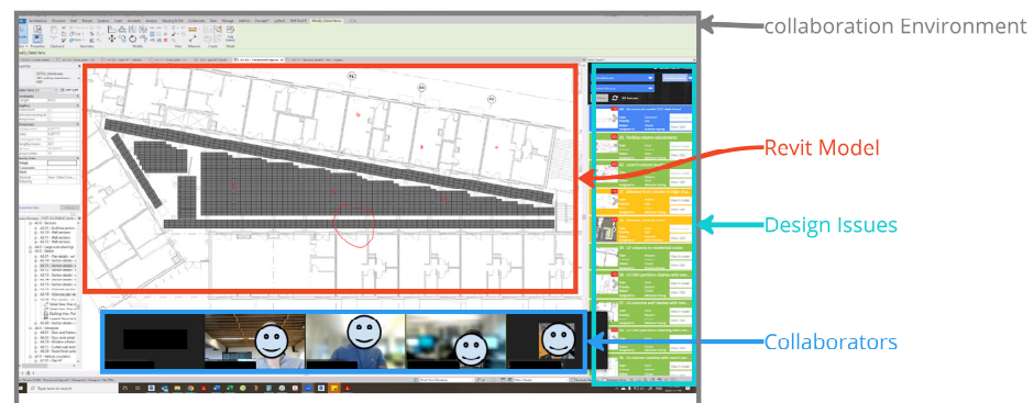
Figure 2. Collaborative design issue resolution by the Vienna House project team, with Revit model (red), collaborators (blue), collaboration environment (gray), and design issues (light blue) highlighted.
