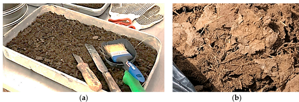
Figure 3. Cow dung dried on pasture after being collected (a) and after manually broken before passing through the electric mill to produce CDdrypow (b).
