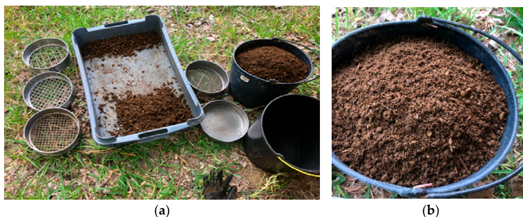
Figure 2. Cow dung sieved after 7 days of drying (a) and after sieving (b).
