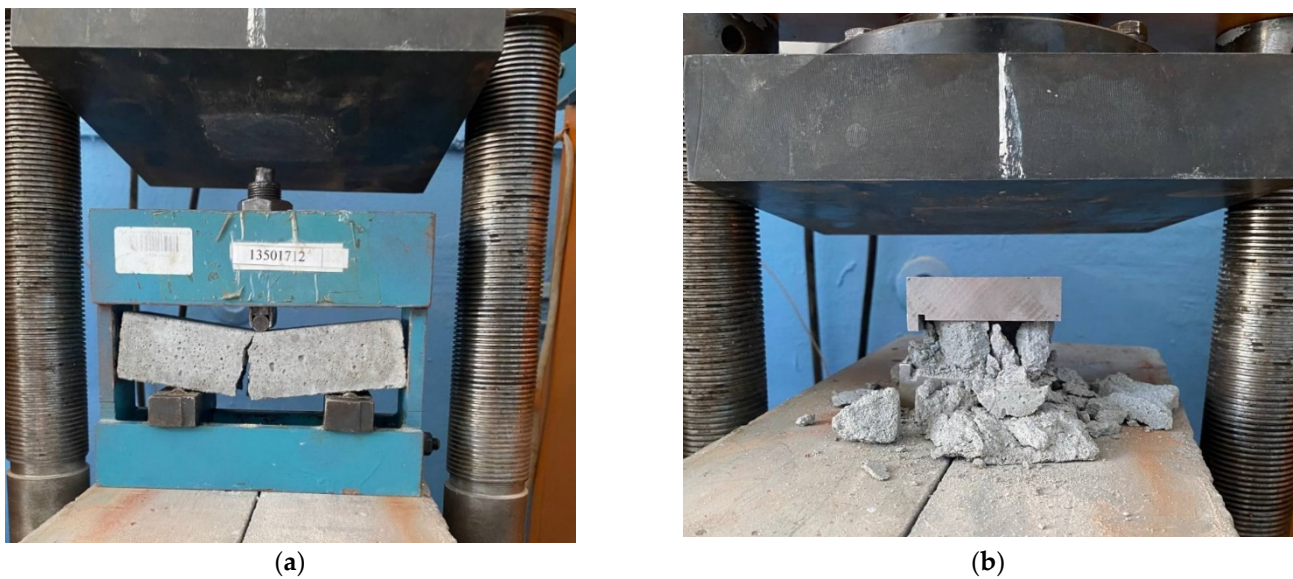
Figure 3. Testing of cement paste samples: (a) flexural strength (b) compressive strength.
