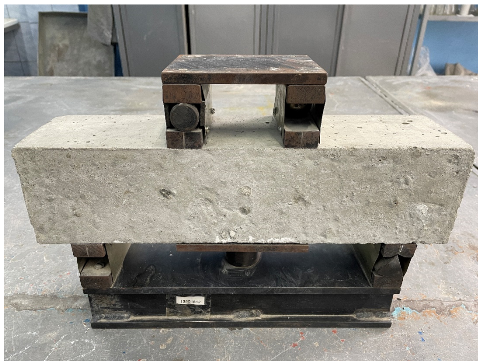
Figure 4. Concrete bending test.
