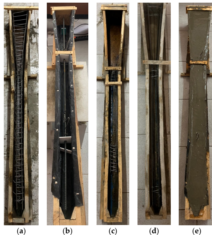
Figure 4. Appearance of pile models and segments filled with fiber-reinforced concrete. Pile Models: (a) SFC-1 and PFC-1; (b) SFC-2 and PFC-2; (c) SFC-3 and PFC-3; (d) SFC-4 and PFC-4; (e) filled with concrete.
