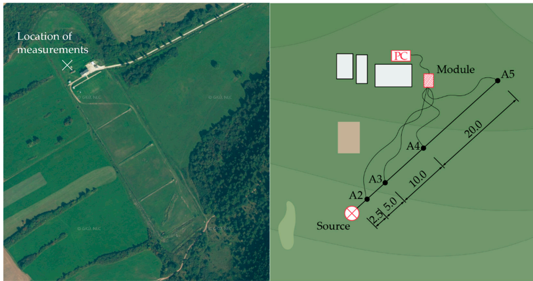
Figure 9. Orthophoto map showing the entire shooting range (left) and a scheme of the measurement setup showing the arrangement of accelerometers in the propagating wave path from the source of the explosion (right).
