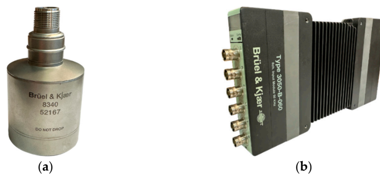
Figure 1. Equipment used for the measurements—accelerometer ( left ) and module ( right ). (a) Accelerometer B&K type 8340; (b) Module PULSE LAN-XI B&K type 3050-B-060.
