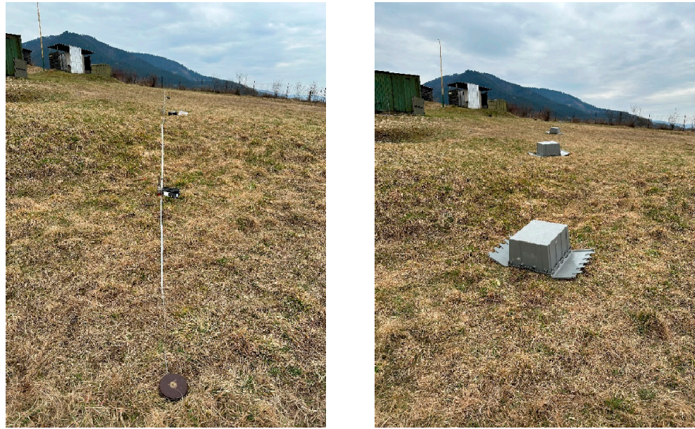
Figure 11. Placement of accelerometers in the direction away from the source of the explosion and in the path of the propagating waves.
