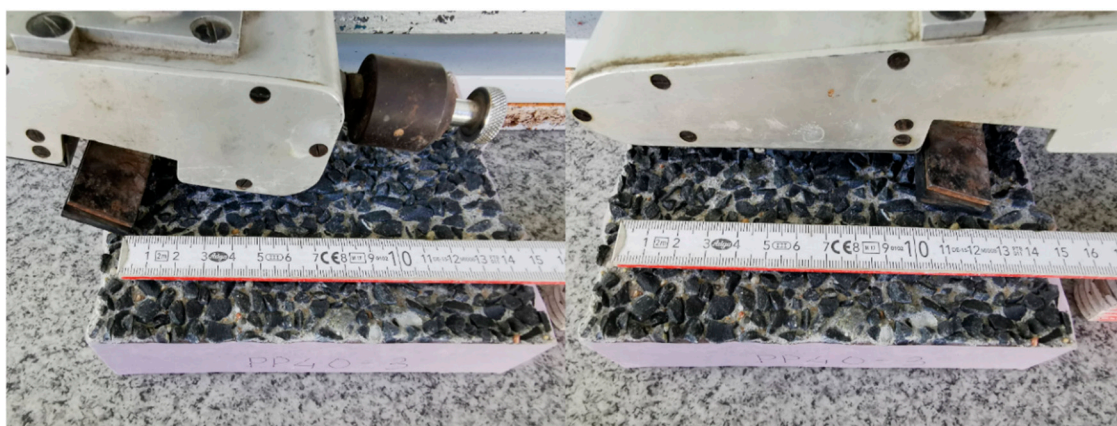
Figure 6. A photograph of a sample with exposed coarse aggregate illustrating the procedure for adjusting the sliding path length for the pendulum test.
