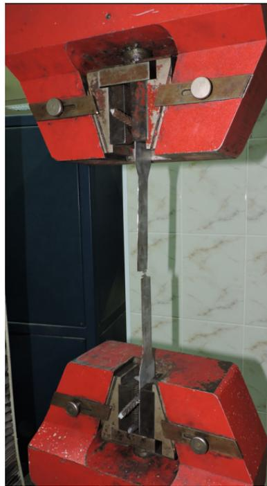
Figure 3. Tensile coupon test of a typical stainless steel plate specimen.
