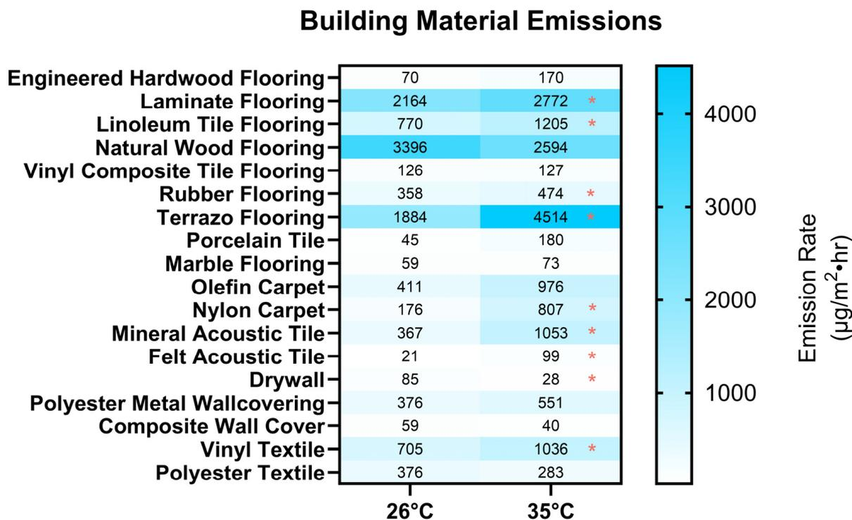
**Figure 2.** Average TVOC emission rates of 18 modern building materials at two studied temperatures. The \* denotes significant change ( $p < 0.05$ ) in emission rate between the two temperatures. Within each material grouping type, the heatmap is organized by increasing price.
