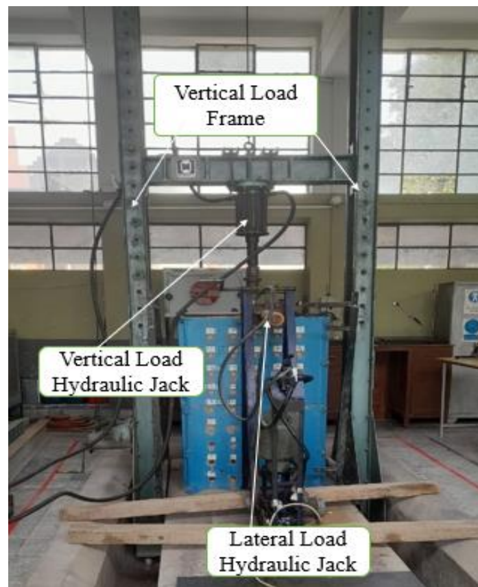
Figure 17. Vertical load setup.
