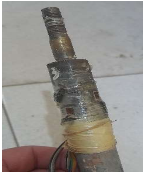
Figure 10. Strain gauge installation.
