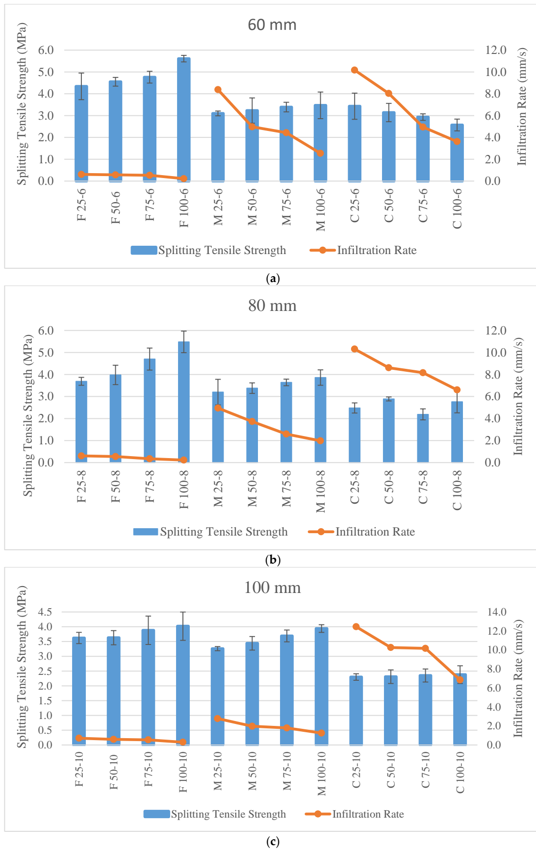
Figure 7. Changes in splitting tensile strength and infiltration rate values of pervious block samples with (a) 60 mm thickness, (b) 80 mm thickness and (c) 100 mm thickness.
