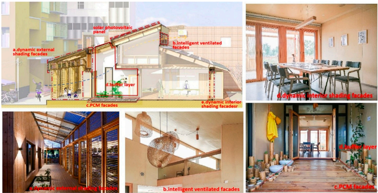
Figure S2 The dynamic facades of the nearly net-zero energy Solar Decathlon house: (a) dynamic exterior shading; (b) intelligent ventilated; (c) PCM facades; (d) buffer layer; and (e) dynamic interior shading facades.
