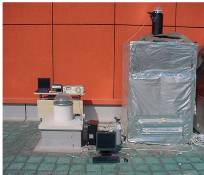
Figure 3. Light pipe-natural ventilation system experimental apparatus.
