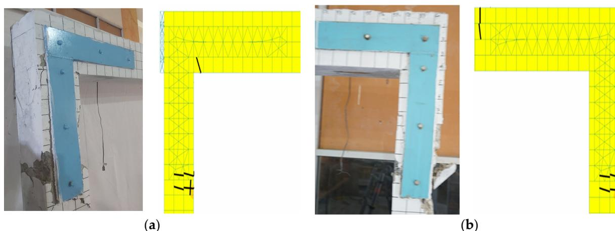
**Figure 10.** Damage observed in NEB-100, (a) right joint and (b) left joint.
